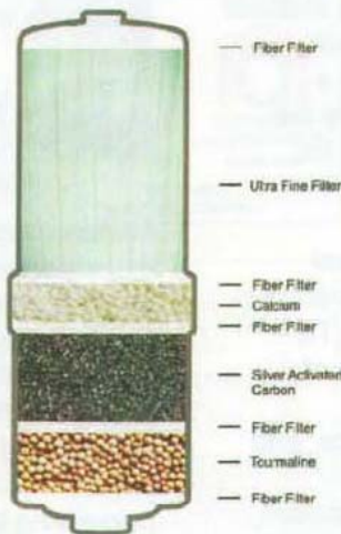
Above is an example of an ionizer internal filter containing alkaline rich minerals; in this case it is Tourmaline.
